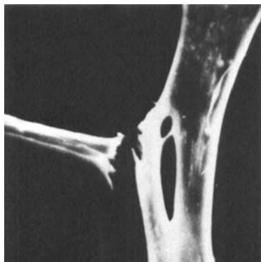
Fig.2 SEM picture of stress cracked fibers of polyacetylene
